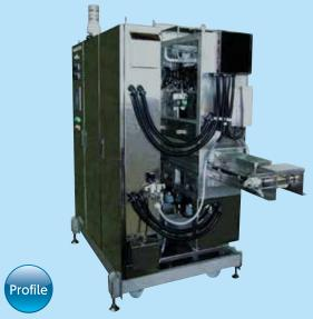
Processed material on the conveyor is heated momentary when it passes in microwave heating cavity.
