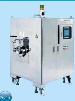
Forming (molding) Pipe is installed in the Microwave heating cavity and filled pasted meat in the pipe is formed to the shape freely.
